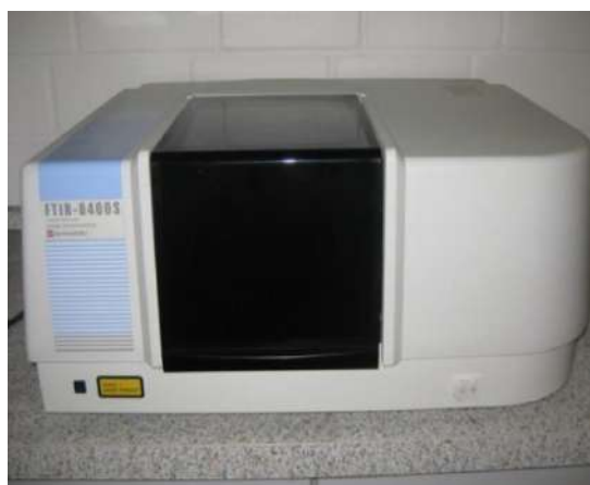
Fig 6: Shimadzu-8400 Fourier transform infrared system
